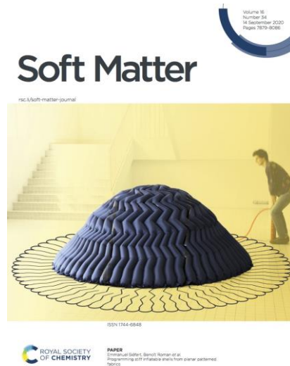
Fig. 1. An inflated planar pattern leads to a dome shape when inflated.
